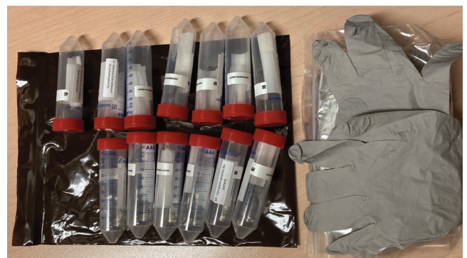
Figure 1. Kit de pr l vement des surfaces EXPOPROF
