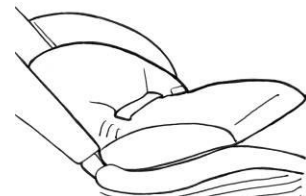
Figure 158. Booster seat (articulated cushion) with a back rest that fits into the dental chair, making it possible to bring the patient's head to the edge of the chairback.
