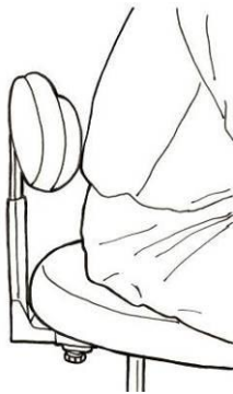
Figure 80. This lumbar support cannot be moved forward, so it is not in contact with the lower back during dental procedures in the oral cavity.
