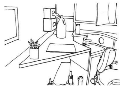
Figure 133. A counter or table on the dominant side to allow taking notes without twisting the body.
